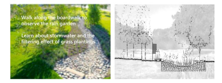
*Purpose:* To show how a rain garden containing grass and other plants work together to retain and filter storm water
