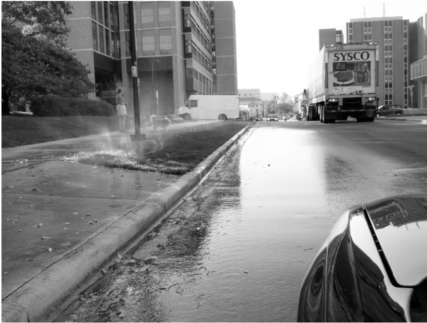
Figure 3-2. Impervious surfaces collect and channel runoff from irrigation or precipitation to storm drains and surface waters, Madison, WI, 2007.
